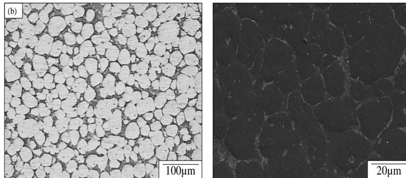
Figure 7. Optical and SEM morphologies of thixoformed-T6 Al-5.7Si-2Cu-0.3Mg alloys
