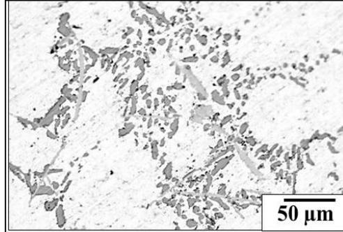
Figure 5. Optical micrographs of thixoformed Al-5.7Si-2Cu-0.3Mg alloy under T6 heat treatment.
