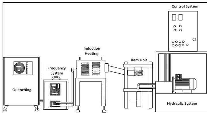
Figure 2. Photograph and schematic of pneumatic thixoforming unit.
