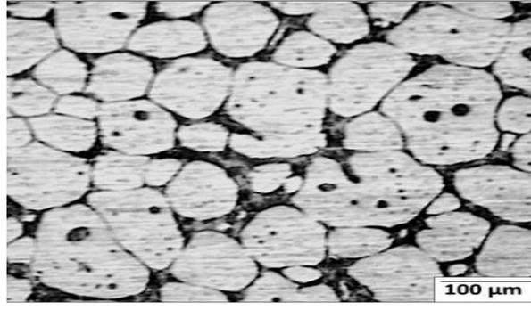
Figure 6. Microstructure of Al-5.7Si-2Cu-0.3Mg alloy after isothermal heating at a liquid fraction of 35% for (a) 3 min and (b) 5 min.
