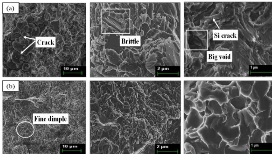
Figure 9. SEM fractographs of (a) as-cast and (b) thixoformed-T6 of Al-5.7Si-0.3Mg alloys.
