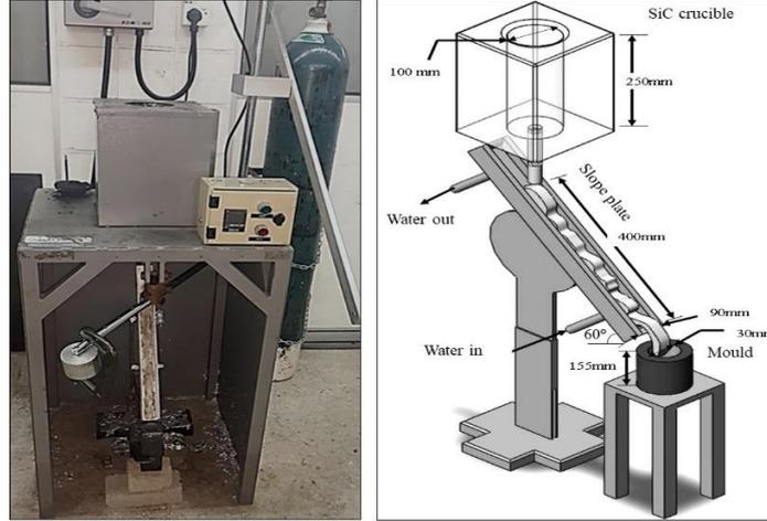
Figure 1. Photograph and schematic of cooling slope casting apparatus.
