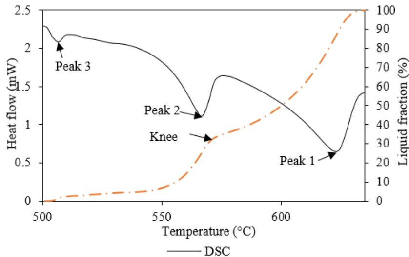
Figure 4. Fraction liquid vs. temperature from DSC graph.
